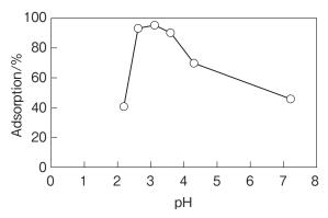
Fig. 1 Effect of pH on adsorption of CBB.
