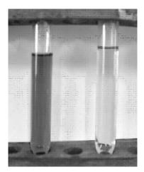
Fig. 4 The photograph of the CBB adsorption test. Left: CBB solution, Right: after removal of CBB
