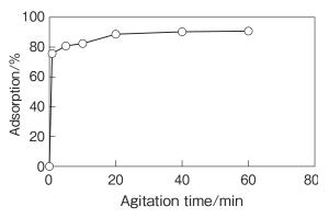
Fig. 3 Effect of agitation time on adsorption of CBB.
