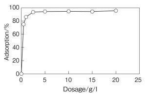
Fig. 2 Effect of the dosage on adsorption of CBB.
